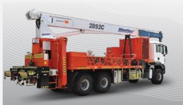
Wireline Crane Truck Unit
