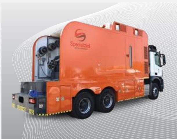
Open / Cased Hole Logging Truck Unit
